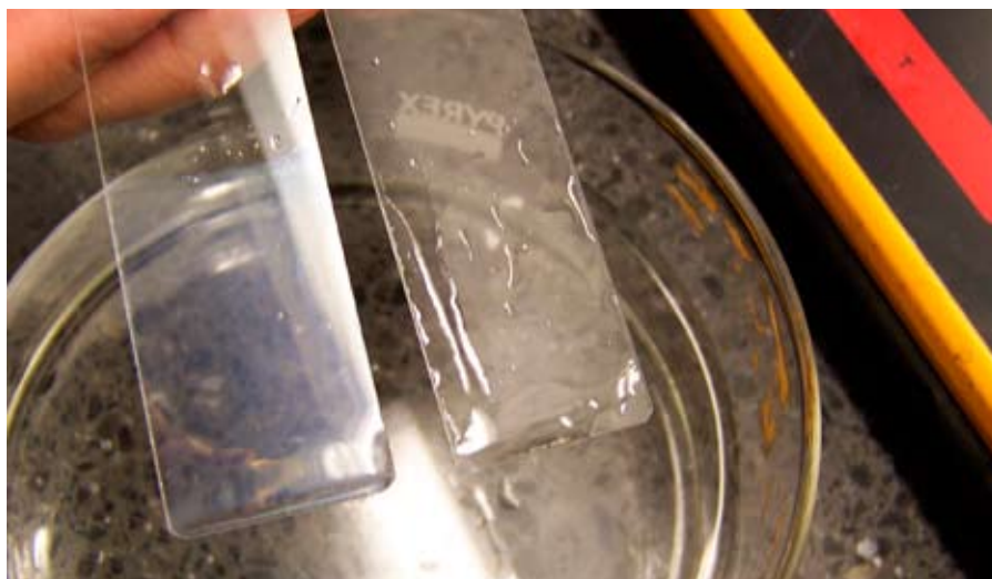
\text{TiO}_2 coated glass (left) exhibits superhydrophilicity when compared to uncoated glass (right).
